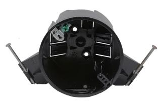
EZ25CNG-HW is a 25 cu. in., nail-on, heavy wall ceiling box for new work (construction) applications for residential and light commercial projects. It is a heavy duty new construction (new work) ceiling box to use where a more durable electrical box is preferred. The harder shell resists flexing and holds shape in extreme conditions. It features 5 heavy-duty wire clamps for EZ secure wiring. It features a ground lug for EZ grounding when required.
